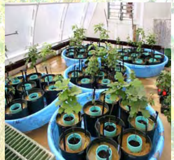
Set-up of experiment showing the pots in which we saturated the soil and the sleeves in which the water was filled to measure the infiltration rate.
